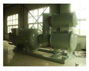
600kV/1.5A SF6 filled Test Transformer for GIS/CVT testing
